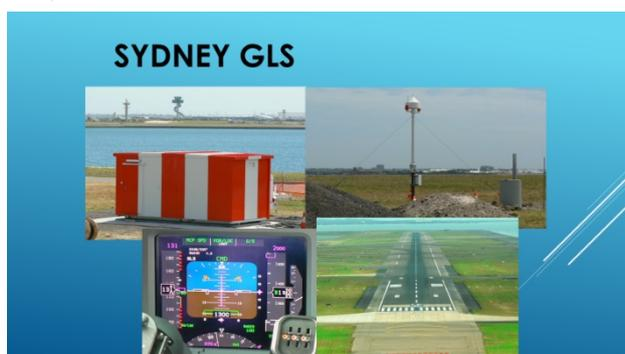
Ground Based Augmentation System Landing System (GLS) can provide CAT I approaches to all runways for appropriately equipped aircraft (normally the larger RPT aircraft) rather than an ILS which is runway specific.
